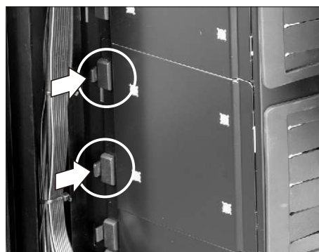
Press to release the HDD tray
