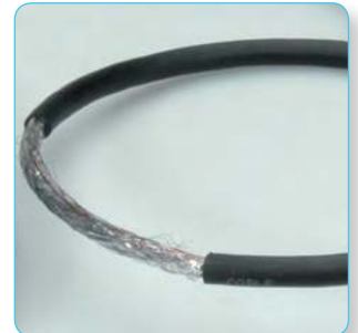
Bad Shielding Cheap Cable
