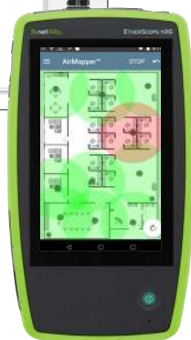
AirMapper Site Survey App on the EtherScope nXG
